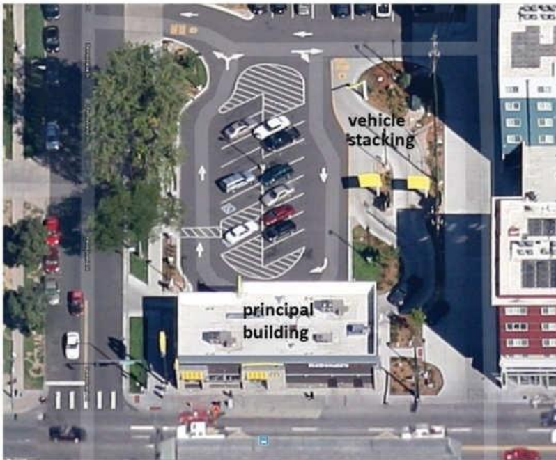
Figure 2332 (6) Recommended Drive-Thru Facility Layout
